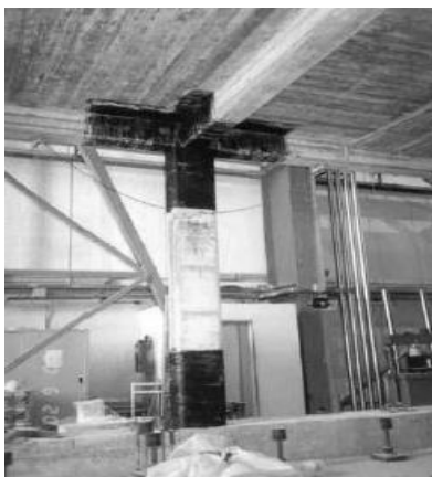
Figure 3. Retrofitting of RC beam-column joints with FRP (Tsonis et al. 2001, Motavalli and Czaderski 2007).
