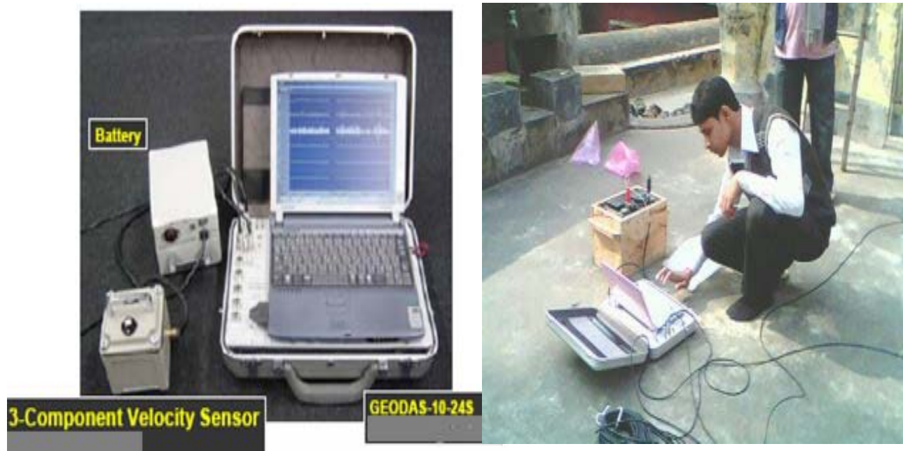
Figure 2. Microtremor equipment with Battery, 3-component velocity sensor and microtremor observation
